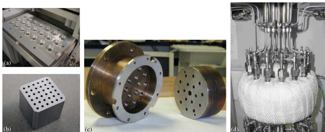
Fig. 4. High-throughput reactors developed at ITQ: (a) 21-batch (liquid/solid) reactor system endowed with a robotic arm for reactant feeding, sampling and injection in a GC; (b) 36-fixed bed reactor system (gas/solid) working at atmospheric pressure and catalyst amount ranging from 5 to 25 mg; (c) 16-fixed bed reactor system (gas/solid) working at atmospheric pressure and catalyst amount ranging from 100 to 1000 mg; (d) 16-fixed bed reactor system (gas/liquid/solid) working at high pressure up to 100 bar and catalyst amount ranging from 100 to 1000 mg.
